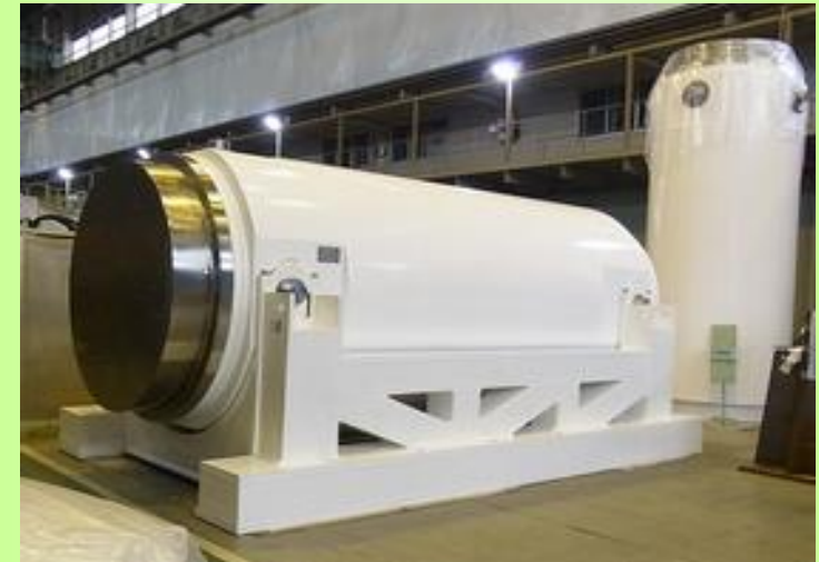
Spent nuclear fuel storage container (Neutron shield material)
