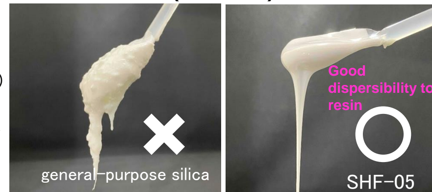
Evaluation of dispersibility to resin of general-purpose silica and the product developed by the company
