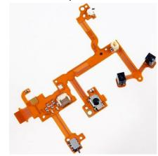
Electronic substrate built in highspeed communication devices
