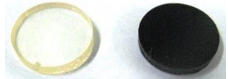
Fluorinated CNT epoxy composite
